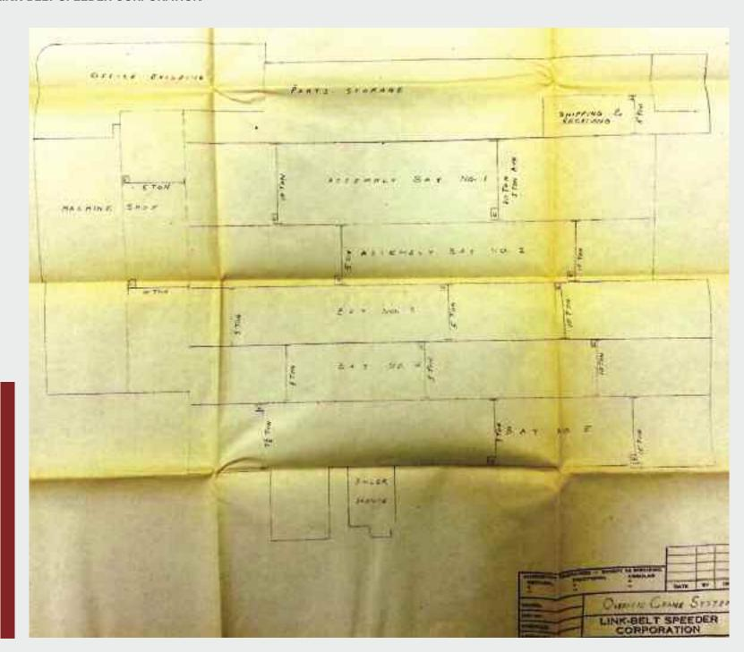
Figure 20. Link-Belt Speeder "Overhead Crane System" Plan showing layout of new plant completed in 1948. Exhibit III From Plant Study, Link-Belt Speeder Corporation, State University of Iowa Thesis by Jerome Greenberg, August 4, 1948. From University of Iowa Special Collections.
