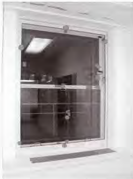
Fig. 8. Interior view of the repaired window prior to installation of the interior chamber. Note the thermal and relative-humidity sensors are indicated with dots. Some sensors are installed on the repaired window, and others are installed on the storm sash, resulting in more sensor locations than on the replacement window.
