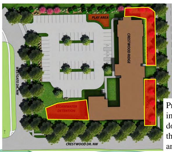
Proposed storm water improvements will decrease downstream runoff through the use of detention basins and infiltration measures.
